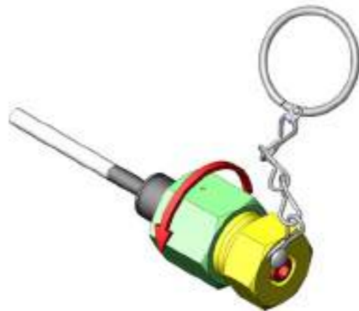
3. Assemble the nut with the plug, then tighten slightly with fingers.
