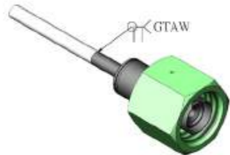
1. Assemble the nipple with the nut, then butt-weld with the tube.
