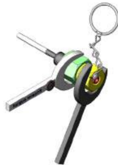
4. Please use the torque wrench to tighten the nut, and torque value of different gaskets can be set as below.
